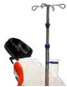
I.V. Pole stainless steel Ø 25 / 18 mm, one-hand height-adjustable 1070-1660 mm, 4 hooks, max. 2 kg 8.4 lbs/hook, glass and holder Item No.: 3068 0000
